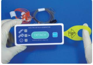
Pull off the POWER ON ribbon and the EDG v4 is powered on.
